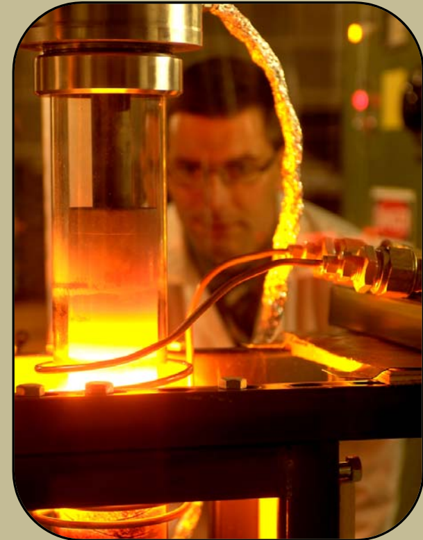
Dr. Travis Knight, co-principal investigator of both USC Nuclear CoEEs, works on a fluidized bed chemical vapor deposition coater to produce coated particle fuels for high temperature gas-cooled reactor applications.
