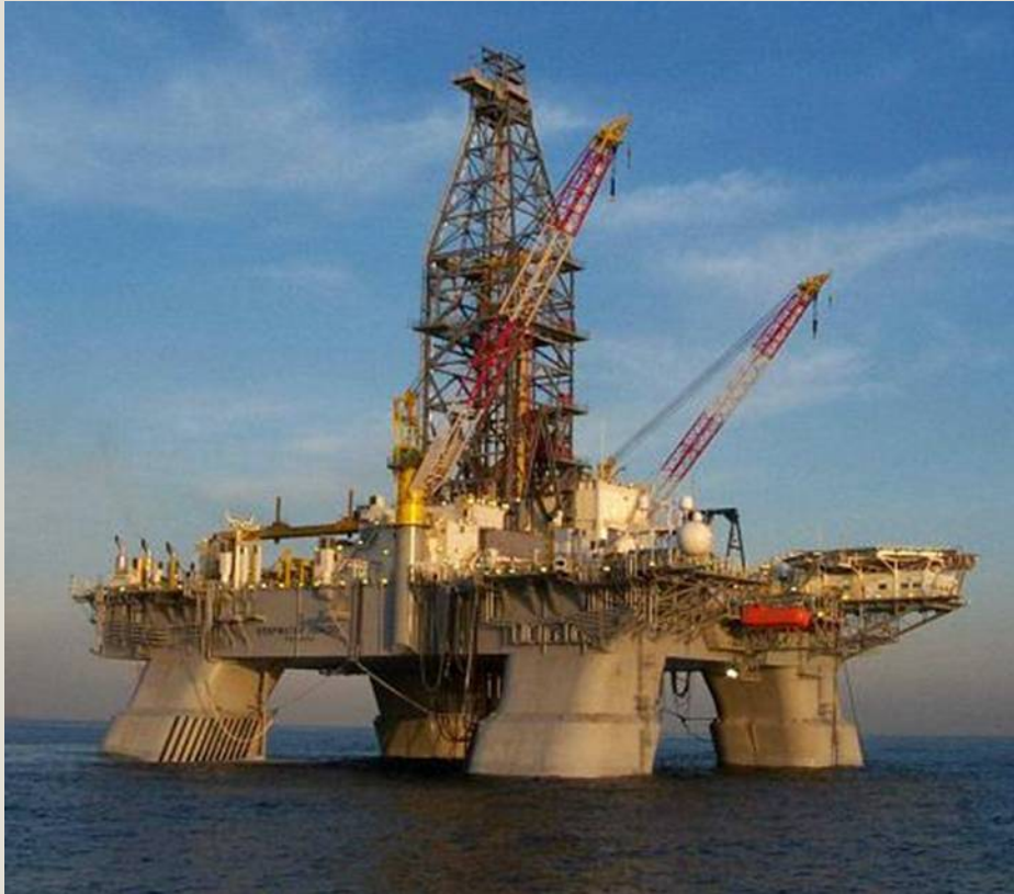
The Deepwater Horizon , a dynamically positioned, semisubmersible drilling unit (photo courtesy of Transocean).
