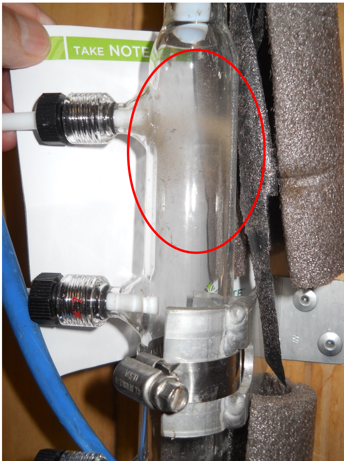
Figure 4: Manifold at Greenville ESC site with residue inside manifold circled.
