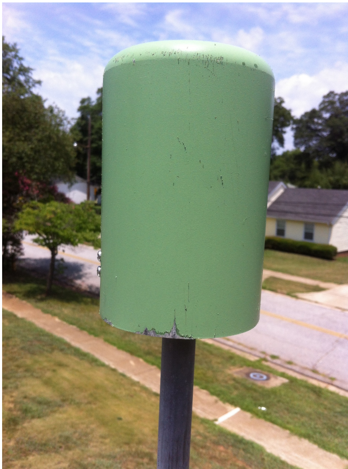
Figure 1: Probe Cap at Greenville ESC Site showing abrasion.
