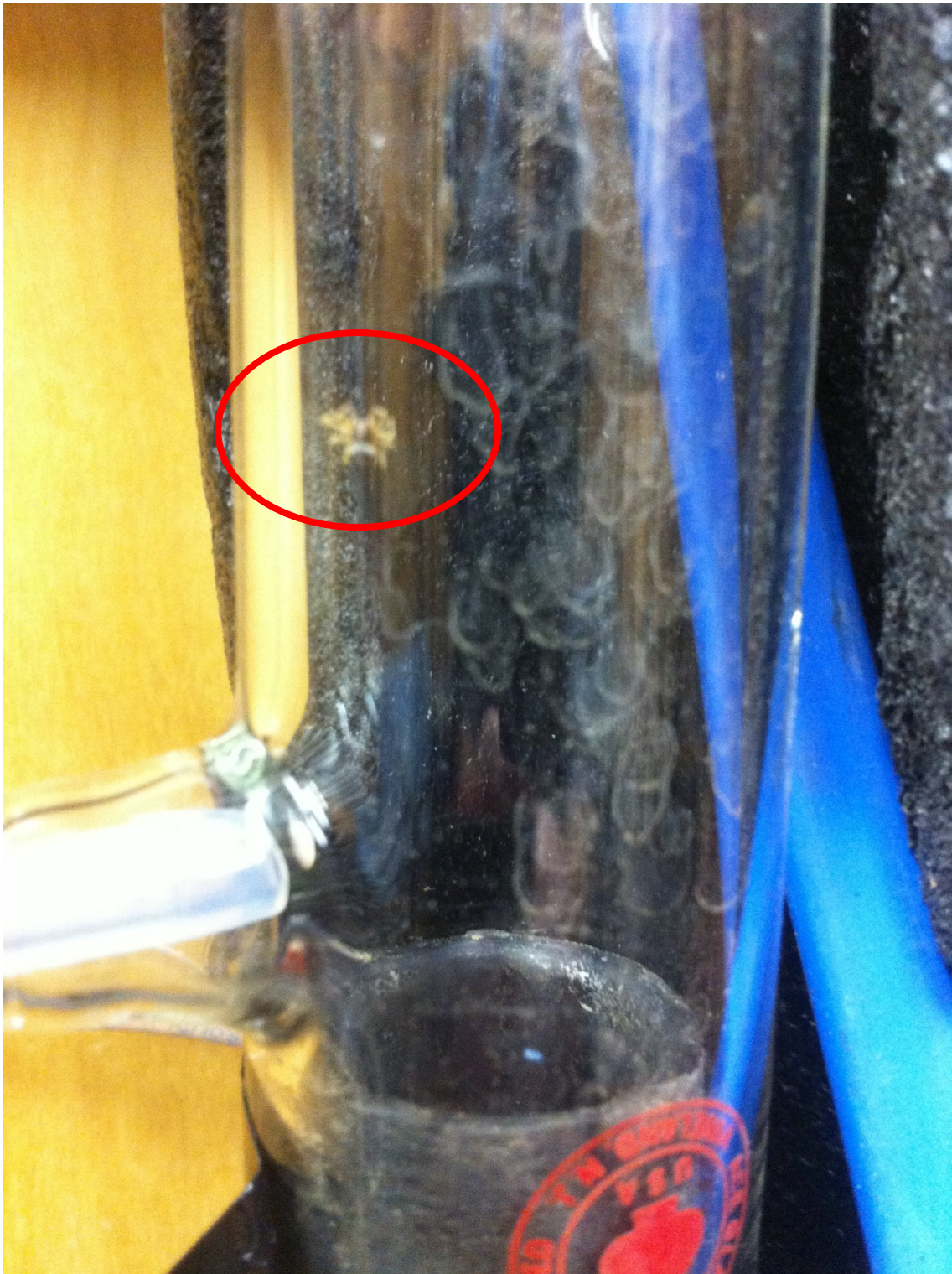
Figure 3: Manifold at Long Creek site with residue visible. There is a spider inside the manifold (circled).
