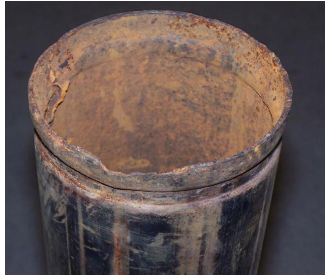
Coastal-Empire MHC corroded sprinkler system pipes. The sprinkler system was installed in 1994 during the original building construction. There have been numerous leaks in the first floor area over the past few years. This system relies on compressed air to function. Loss of air pressure from corroded piping results in frequent activation of the air compressor. Compressor noise reverberates up through the second floor. A study by MECA, Inc. identified numerous deficiencies from the original installation including improper sloping of the dry pipe system and lack of adequate auxiliary drains.
