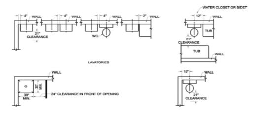
FIGURE 307.2 MINIMUM FIXTURE CLEARANCES
